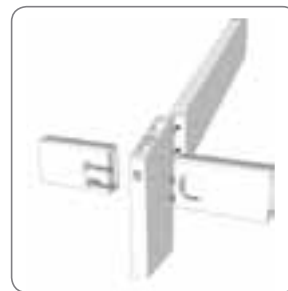
Eaves purlin - exploded view
